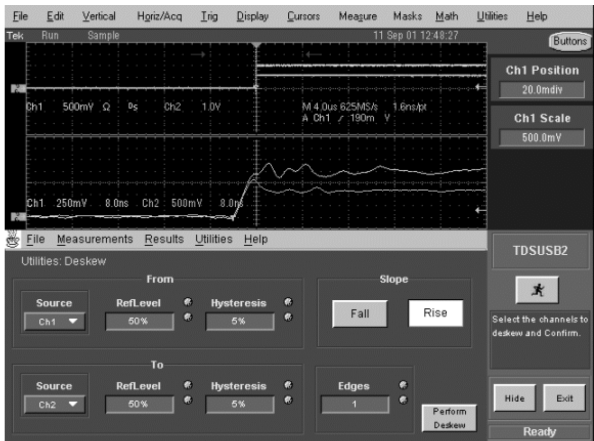
Figure 1-2: Signals after the single edge deskew
